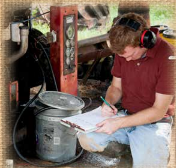
Staff monitor fuel usage during a pumping plant efficiency test.
